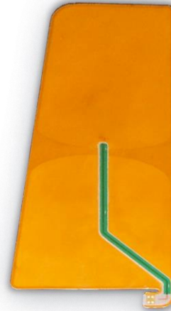
Flexible “Peel-And-Stick” Dipole Antenna
